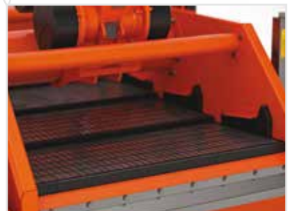
Largest non-blanked screen area among shakers of similar footprint: 21.2 ft 2 (1.97 m 2 )
