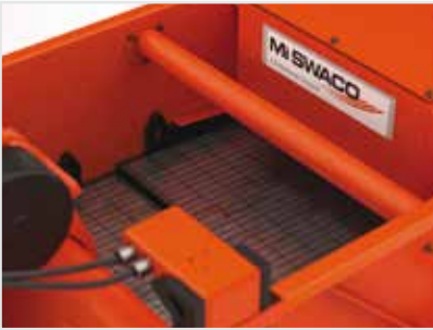
Increased access for inspection, installation, and removal of screens
