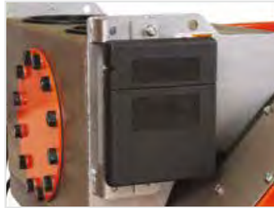
Patented high capacity distribution box with low weir height
