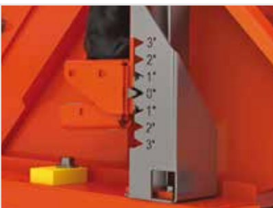
Deck angle can be adjusted while processing fluid. Adjustment Range is -3° to +3°
