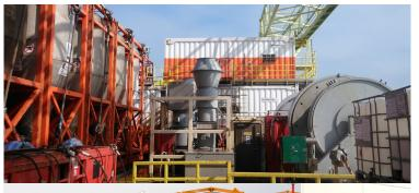
A total of 2,968 tonUK of oil-based cuttings was treated on the rig and discharged with average TPH of less than 0.1%, significantly lower than the 1% regulatory limit, with zero NPT. Additionally, 2,870 bbl of base oil valued at USD 348,000 was recovered for reuse and an estimated 3,600 offshore crane lifts were eliminated.
