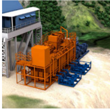
Heliportable rig in the jungle featuring modular CRI equipment
