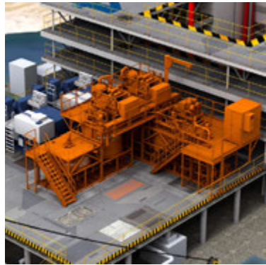
Offshore production platform with space-optimized CRI equipment
