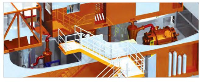
The HAMMERMILL unit is specifically designed for offshore, capable of being installed in the space that would have been used for the skips previously used to collect and transport cuttings to shore.
