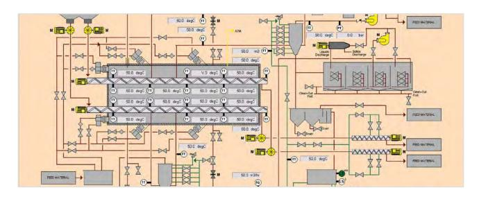
M-I SWACO THERMAL PHASE SEPARATION (TPS) technology delivers an unprecedented level of economy and environmental benefits in the treatment of drilling fluids and drilled cuttings. These systems provide a completely self-contained, versatile process based on indirectly heated thermal desorption.
