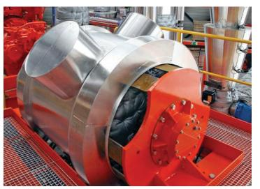
The process mill is the heart of the TCC HAMMERMILL system. Recovered base oil is transported back to the liquid mud plant for reuse in the formulation of new and reconditioned OBM. The treated solids have an average TPH of 0.2%. To date, the system has treated more than 200,000 t of OBM cuttings and recovered more than 150,000 bbl of base oil for reuse.
