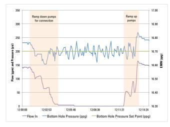
Figure 2: Response of the MPD system during a connection
