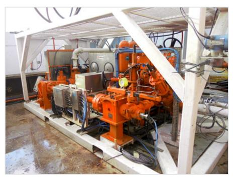
Figure 4: @balance Services DAPC choke manifold
