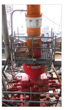
Figure 5: HOLD RCD on top of annular preventer
