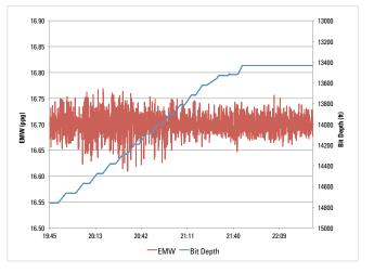
Figure 3: Near-constant bottomhole pressure while stripping out of hole
