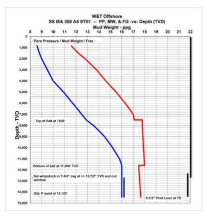
Knowing the challenges that could be faced drilling through such a narrow mud weight window, W&T Offshore chose to employ a proactive MPD approach by using the @balance Services DAPC system to automatically manage the wellbore annular profile.
