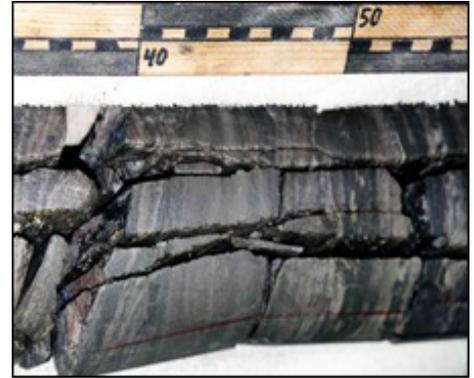
*The reservoir formation was highly fractured, held cavities, and was extremely prone to swelling under high mud column pressure.*
