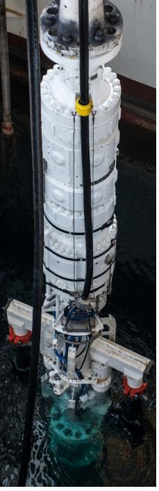
Below tension ring rotating control device.
