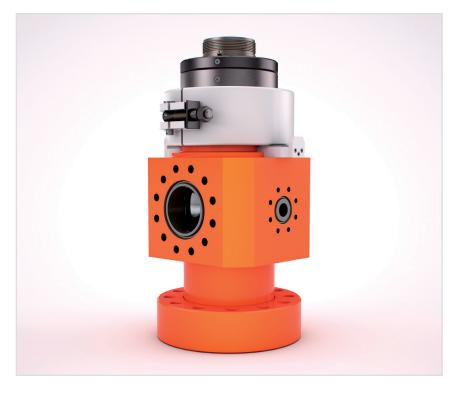
The RCD 3 is the most compact-designed RCD in the industry with a sealed bearing assembly. A complete equalization loop is included with the package along with a remotely operated hydraulic valve located on the 7%-in side outlet. The rig crew can be trained to operate the RCD independently.
