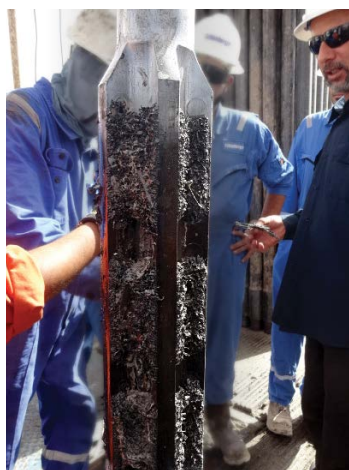
The design of the MAGNOSTAR magnet maintains sufficient flow around the tool during the debris-capture operation.
