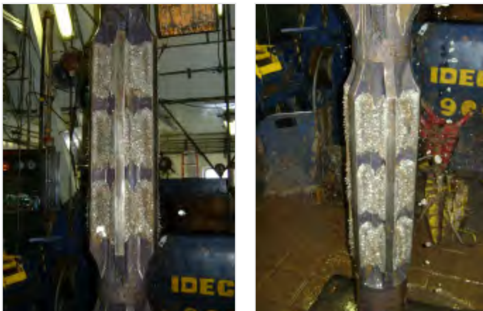
MAGNOSTAR tools loaded with debris
