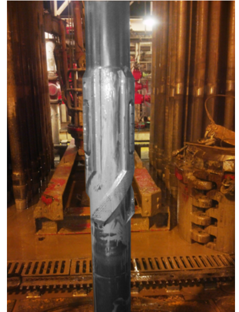
The scraper blades of the SWITCHBACK SCRAPER cleaning tool are retracted to run in hole.
