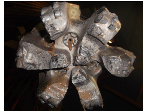
A severely damaged PDC bit was not able to reach TD and created debris downhole. The MAGNOGARD and MAGNOSTAR magnets recovered 44 kg of debris that would have caused further complications to drilling operations had it remained downhole.
