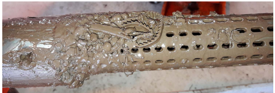
The MUDGARD filter captured several large pieces of ferrous debris.
