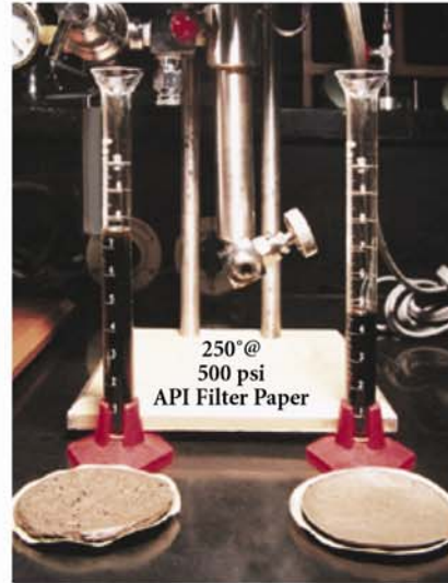
BEFORE AFTER HTHP FILTRATION TEST Note the filtrate reduction after Black Fury.
