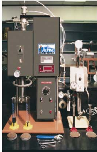
ALPINE MUD PRODUCTS DYNAMIC FILTRATION AND HTHP FILTRATION TEST EQUIPMENT
