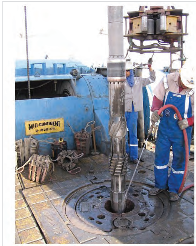
WELL COMMISSIONER tool emerging from Inflow Test and clean-up in Saudi Arabia, after the cement and shoe track had been drilled on the same trip
