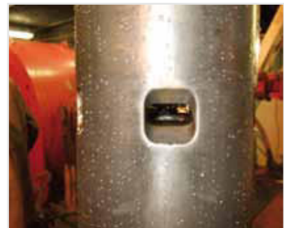
Open circulating ports provide generous flow area
