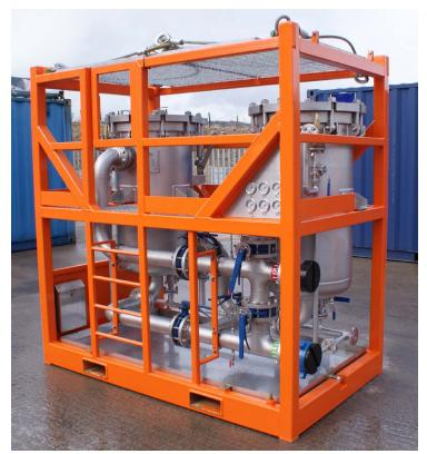
Featuring a reduced footprint, the compact dual-vessel filtration unit does not need additional filtration equipment for further fluid processing.
