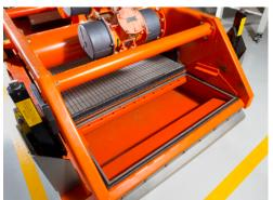
Compared to similar wells with conventional vertical dryers, the SCREEN PULSE separator reduced mud on cuttings by 36% and returned a significant amount of drilling fluid to the active system. This saved more than USD 237,000. Waste was reduced by 420 tUS.
