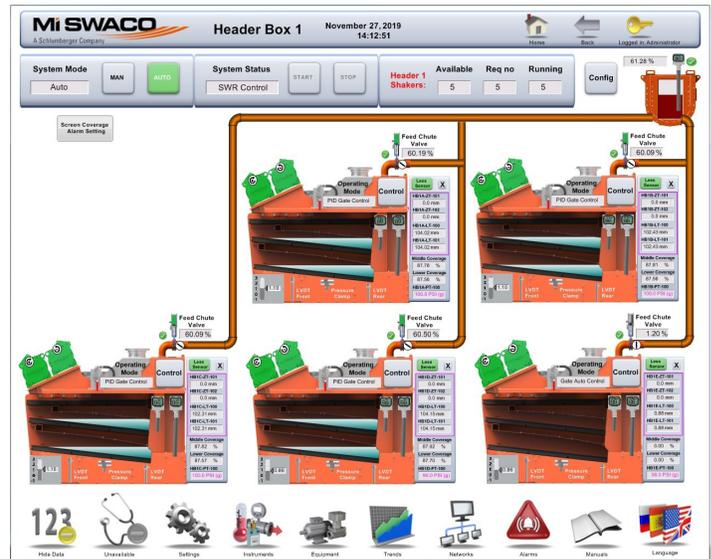
*The full automation package expands the functionality of MD-3 shakers to include remote control from a safe area as well as fully automatic controls to minimize exposure of personnel to the hazardous area.*
