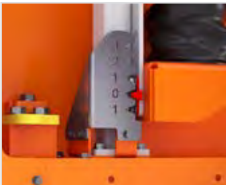
Deck angle can be adjusted while processing fluid . Adjustment Range: - Scalping deck: -1^{\circ} to +3^{\circ} - Primary deck: +3^{\circ} to +7^{\circ}
