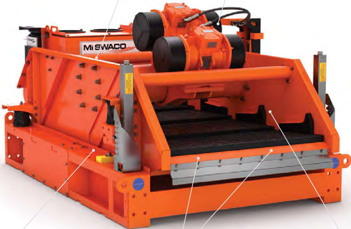
Increased access for inspection, installation, and removal of screens
