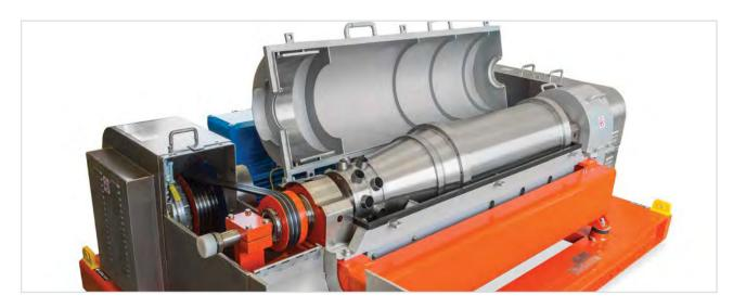
The 518 High Volume (HV) centrifuge is a unit which replaces the operation of two standard 518 centrifuges combined through an increased fluid handling capacity and improved solids separation.
