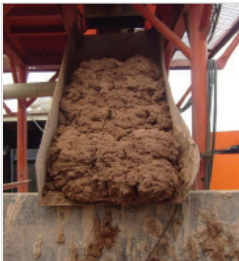
Figure 4. Solids discharge of the M-I SWACO 518 HV CENTRIFUGE
