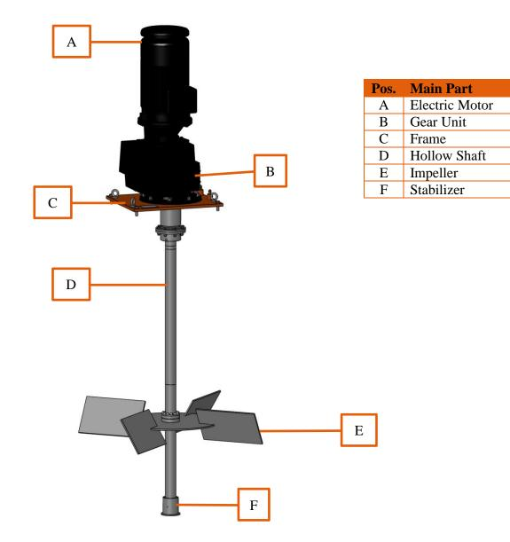
An explosion proof electric motor is connected to a gearbox to drive the impeller shaft (shown in the figure) with required speed and torque. The impeller rotation generates homogeneous mud mixing.
