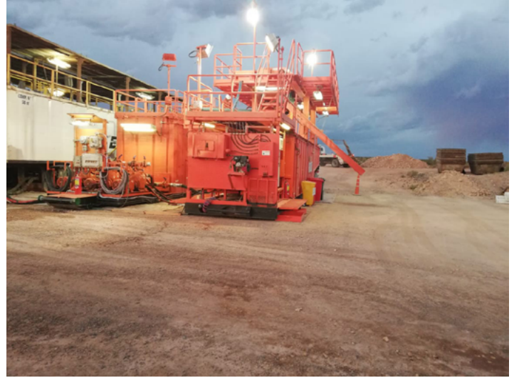
The offline mud treatment on several horizontal wells successfully cut LGS from >10% to <3%.
