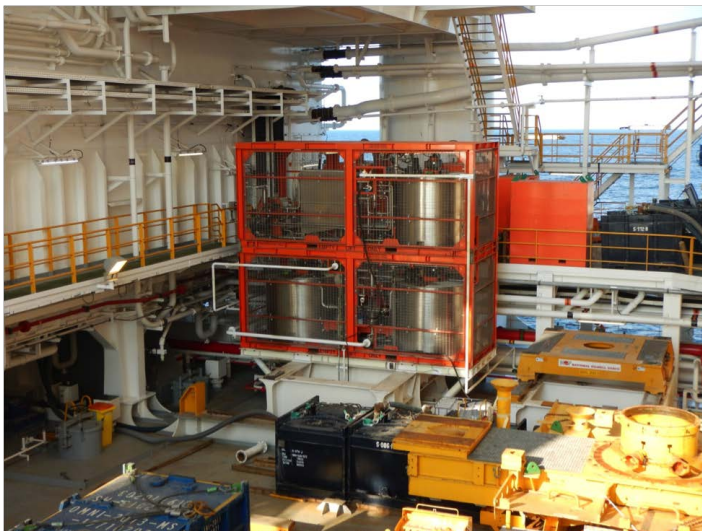
The compact ENVIROUNIT system reduces costs of onshore disposal while meeting discharge regulations. The unit treated 16,500 m 3 of slop water offshore Republic of the Congo, recovering approximately 315 m 3 of synthetic-base drilling fluid for reuse in the active mud system. Only 530 m 3 of waste was sent to shore for disposal.
