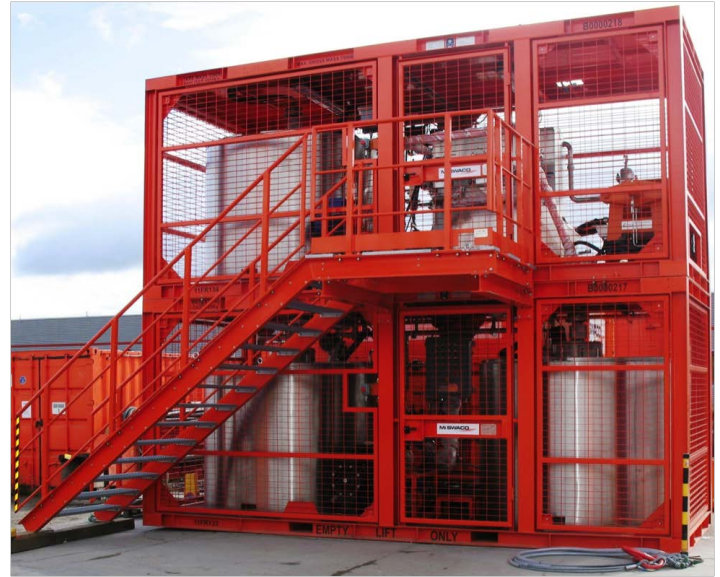
The ENVIROUNIT system provides a rig-based, modular solution for treating and recycling waste and recovering drilling fluid at remote deepwater wells.
