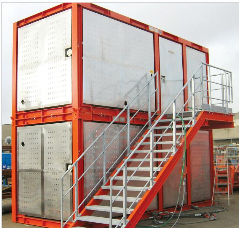
With the petroleum industry moving toward zero discharge from offshore installations, there is a growing need for rig-based, purpose-built, modular units that can treat and recycle fluid resources that are currently sent onshore for waste disposal. This is particularly important for deep and ultra-deepwater wells far from shore disposal facilities and that rely on enormous volumes of drilling, reservoir drill-in and completion fluids.
